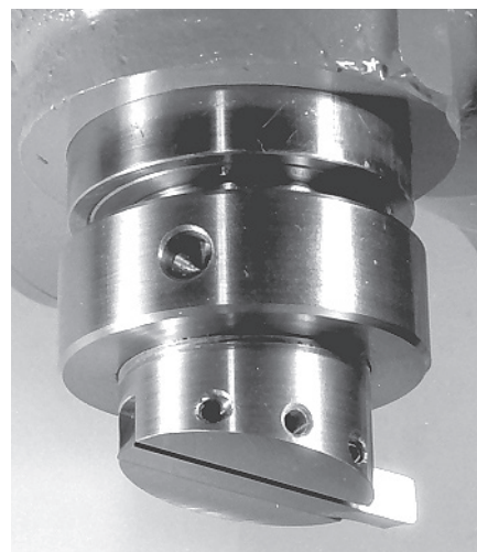
Figure 4 Machining the inner radius of the C-spanner
