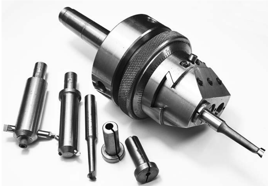
Figure 12 The completed boring and facing head with a selection of tools and sleeves alongside
